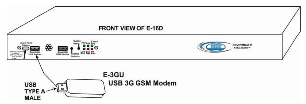
Once installed, the SYSTEM will sense the modem and provide status information on the "Enterprise Configuration" page in the web browser.
