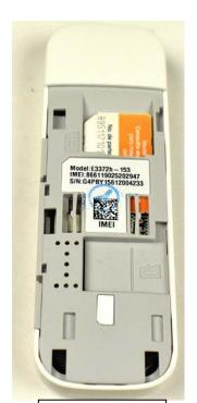
4- Slide SIM card into slot fully. (Card is fully in slot above)
