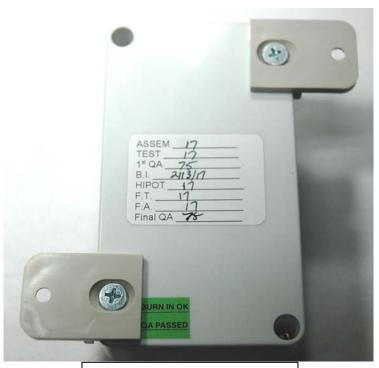
Brackets and screws installed.
